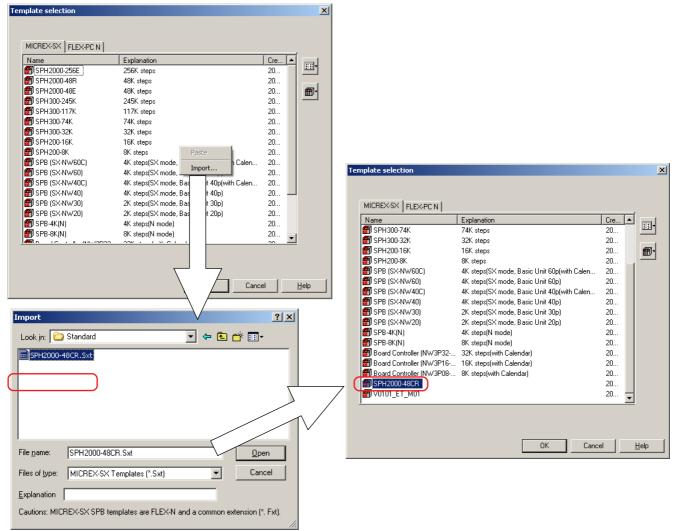
Template of <SPH2000-48CR> is registered at [Template selection] screen.
